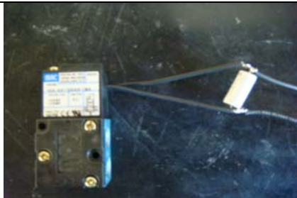
Capacitor shown installed close to the solenoid.
