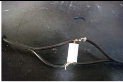
Here it is with solder fully applied to both sides.
