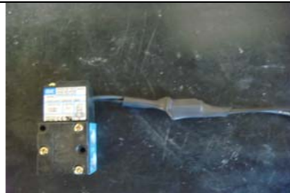
Shown covered with shrink tubing.
